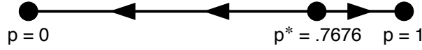
Figure 9.6: The renormalization group flow diagram for percolation on a square lattice corresponding to the recursion relation (9.63).
