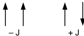
Figure 5.1: Two nearest neighbor spins (in any dimension) have an interaction energy -J if they are parallel and interaction energy +J if they are antiparallel.
